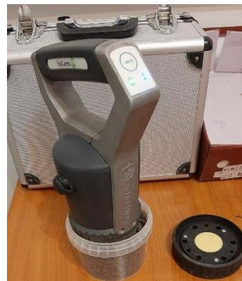
Figure 2. The Soil Cares soil scanner and its use for soil measurement
